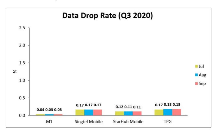
Data drop rate measures the inability of the 4G network to maintain a connection. It may happen because of radio link failures, uplink or downlink interference, bad coverage, unsuccessful handovers or any other reason.
