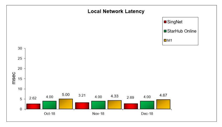
Local latency measures the round-trip time for PING packets to travel between the test clients in Singapore and the Broadband Access Service Provider's ("BASP's") test node(s) in its local Point-of-Presence ("PoP").
