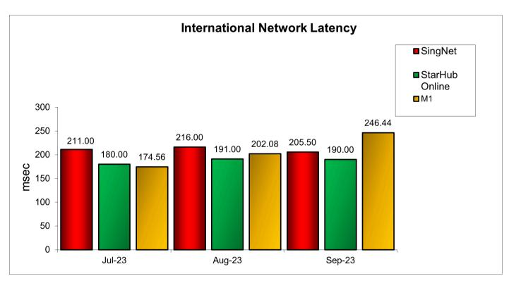
International latency measures the round-trip time for PING packets to travel between the test clients in Singapore and the BASP's test node(s) in its first US PoP.
