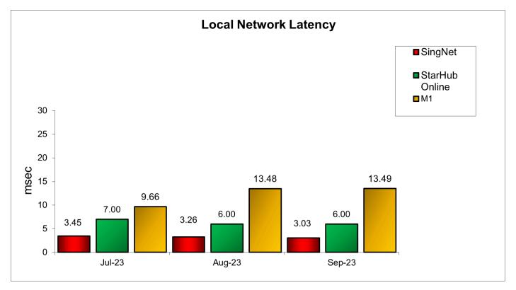
Local latency measures the round-trip time for PING packets to travel between the test clients in Singapore and the Broadband Access Service Provider's ("BASP's") test node(s) in its local Point-of-Presence ("PoP").
