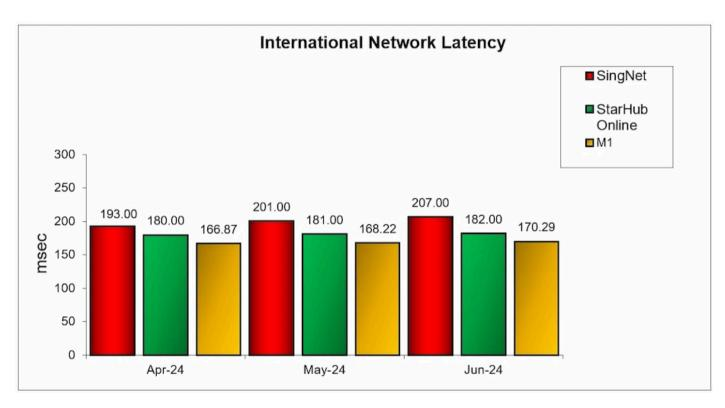
International latency measures the round-trip time for PING packets to travel between the test clients in Singapore and the BASP's test node(s) in its first US PoP.
