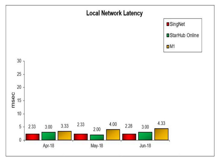
Local latency measures the round-trip time for PING packets to travel between the test clients in Singapore and the Broadband Access Service Provider's ("BASP's") test node(s) in its local Point-of-Presence ("PoP").
