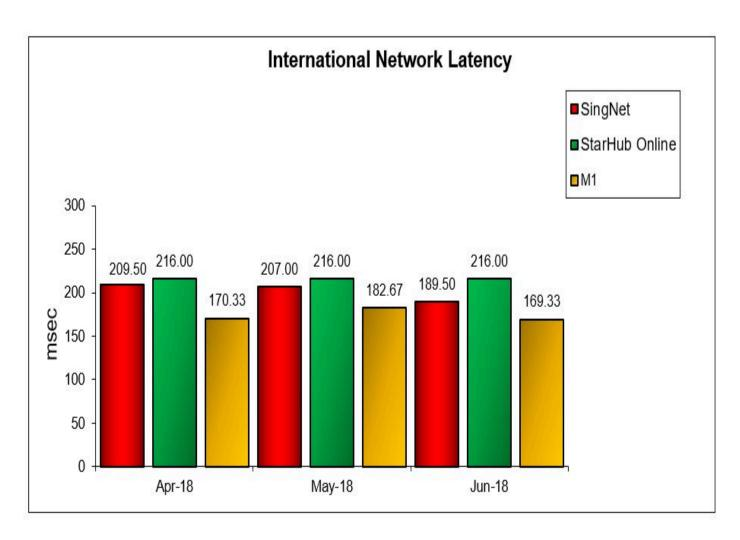
International latency measures the round-trip time for PING packets to travel between the test clients in Singapore and the BASP's test node(s) in its first US PoP.
