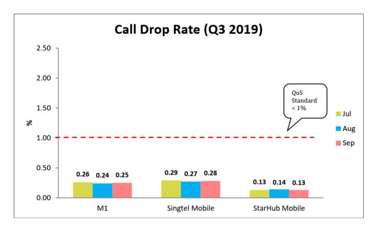
**Note:** Call drop rates are based on the mobile telecommunication operator's actual network traffic logs.
