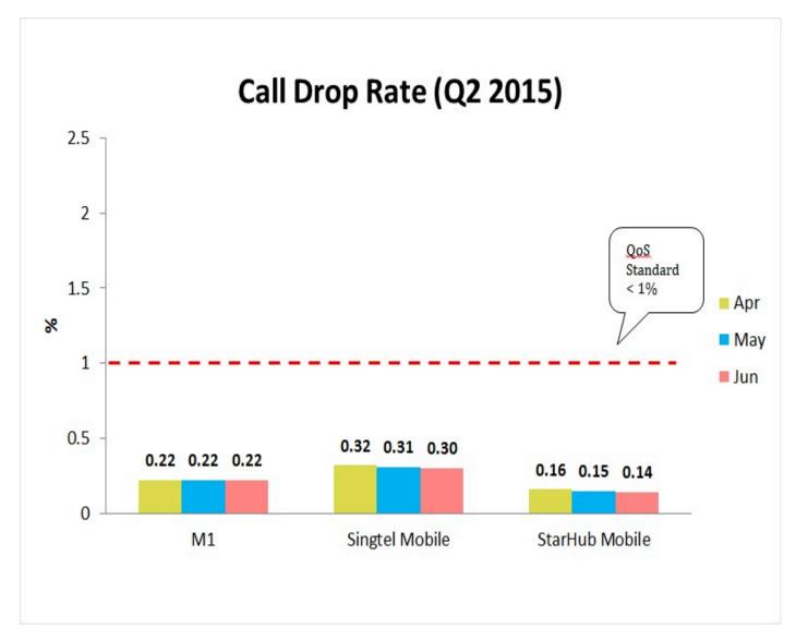
Note: Call drop rates are based on the mobile telecommunication operator's actual network traffic logs.
