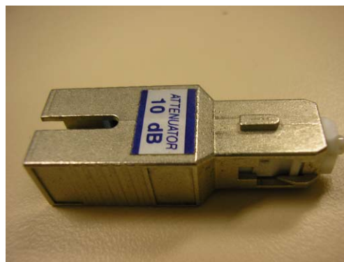
Figure 17: An Optical Attenuator in the Form of an Optical Fibre SC-SC Adapter
