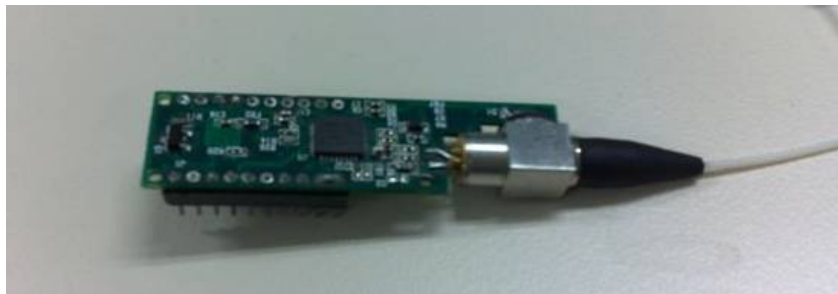
Figure 18: A GPON Transceiver without External Metal Enclosure (Courtesy of A*STAR Institute for Infocomm Research)
