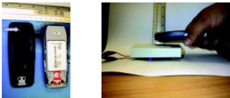
Figure 5. Final placement of chip (left) and testing of chip within interrogation zone (right)
