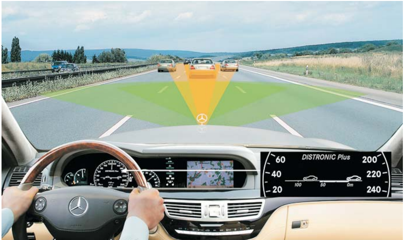
An example of Ultra-WideBand technology – The world's first autonomous intelligent cruise control system using radar-based technology.
